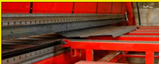
Press brake with digital control
