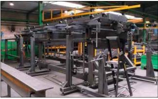
The jigs used in the factory ensure precision and rapidity during the manufacturing process
