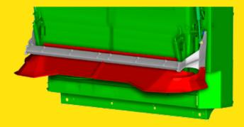
To spread at the field edge, JOSKIN spreaders can be fitted with an independent hydraulically controlled limitation board on the left and/or right.
