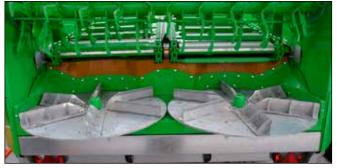
Two wide spreading discs (Ø 1,040 mm) with 6 adjustable blades spread over the width.
