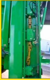
The beaters are driven by P.T.O.shafts (1,000 rpm) and turn at 550 rpm.
