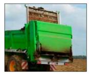
The Ferti-SPACE HORIZON muck spreaders is standard fitted, with a guillotine door. For further information, see page 12.
