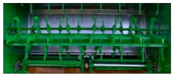
Both beaters with a diameter of 600 mm crumble and shred the matter very well. As a result, the different products are precisely spread.
