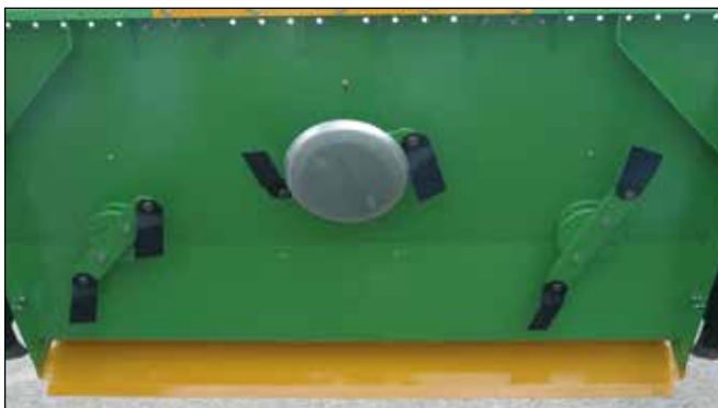
TR pasture toppers are fitted with several small rotors (2, 3, 4 or 2 x 3). Each of them is fitted with a blade holder with two retractable blades of the "TD type" that can turn on 360°
