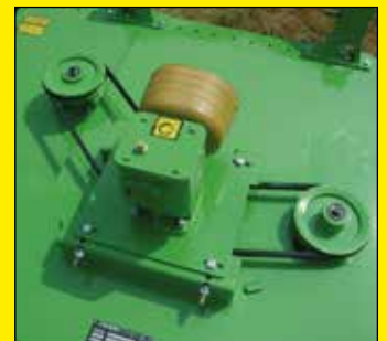
The different rotors are driven by 2 V-belts
