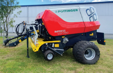
POTTINGER IMPRESS 125F PRO Fixed Chamber baler 32 Knives, 2.3m Pickup Power control/ISOBUS compatible
