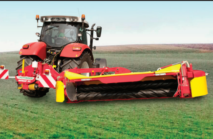
POTTINGER NOVACAT 302 RCB MOWER 3.05m rear vertical fold mower, Roller conditioner model, All gear driven
