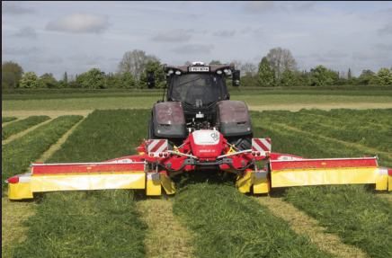
POTTNGER A9 DOUBLE REAR MOWER CONDITIONERS 8.92m Cut, Removable Conditioners Hydraulic Suspension and Break-Away Safety Unique Pottinger Y Drive Gearbox
