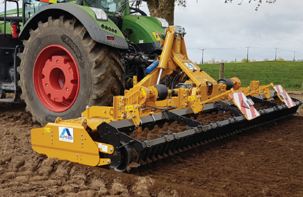
ALPEGO DMAX 5.0m FOLDING P/HARROW 440HP Rated, 520mm Dia packer rollers Drop forged 18mm thick tines Walterscheid drive shafts with cam-clutches
