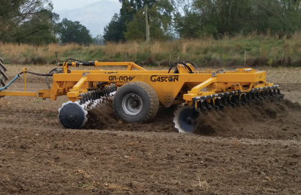
GASCON EOS FOLDING OFFSET DISCS 4.05m and 4.55m Folding Disc Harrows 170-240HP Rated Hydraulic width/Angle/Folding
