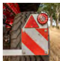
Warning sign with lighting
